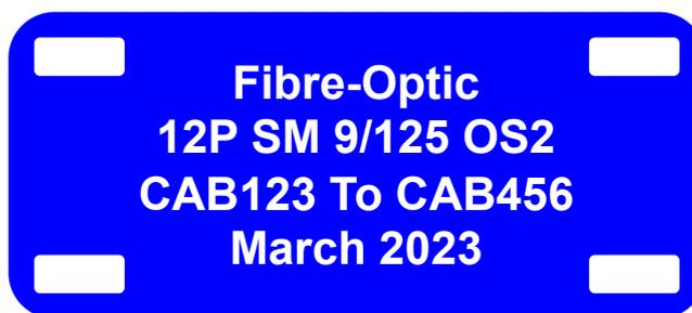
Figure 19: Fibre-Optic Cable Label
