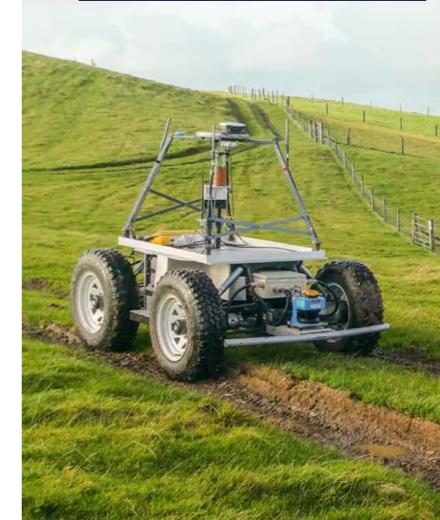
ldris is a four-wheel drive and steering electric vehicle. The main use of ldris is for the Department of Computer Science's research in field robotics and in particular, visual navigation.
