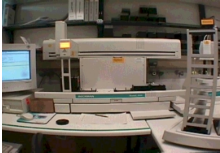
Figure 3: Beckman/Coulter Biomek 2000. A standard laboratory robot designed for liquid handling tasks.
